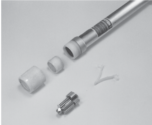
FIGURE 9-2 Twist-grip compression nut lock, cam lock, and tool clip.
