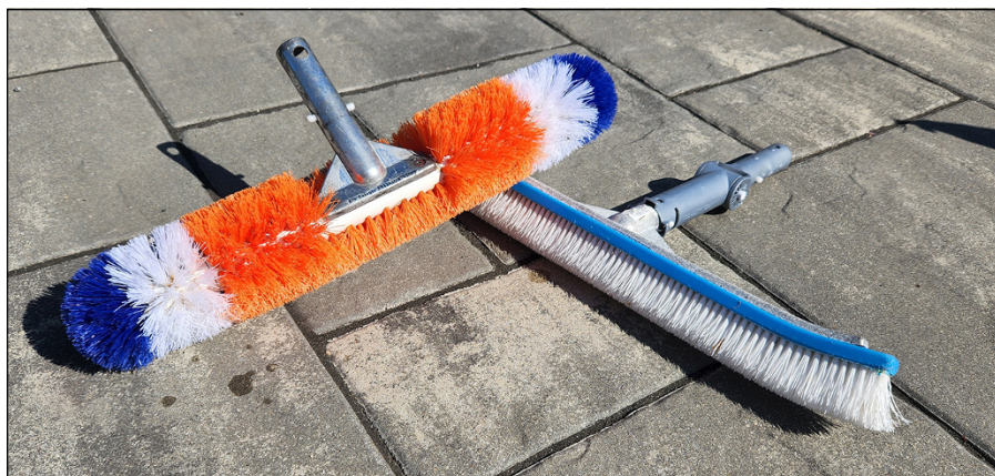
FIGURE 7-7: An example 360° nylon bristled brush and a standard nylon bristled brush.
