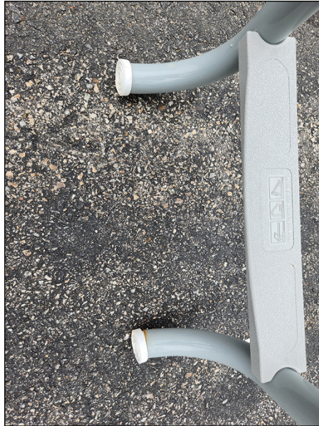
FIGURE 6-7: Ladder bumpers in place.
