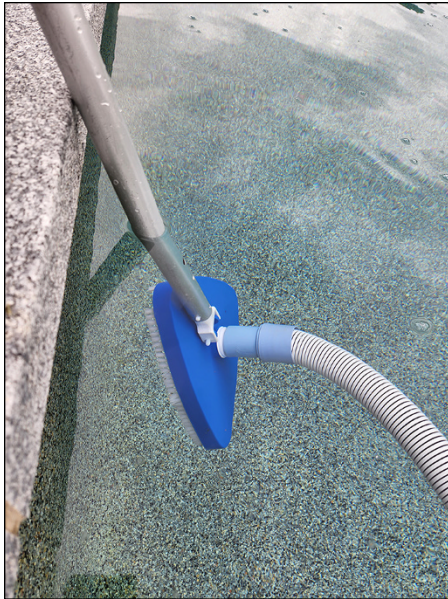
FIGURE 7-4: A vacuum head, pole, and hose submerged under water.
