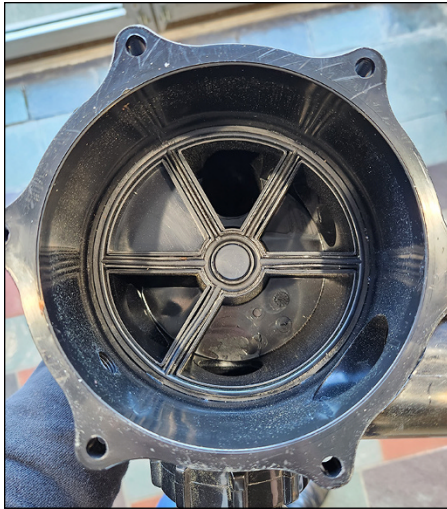
FIGURE 4-2: Inside a multiport valve after the top half is removed.
