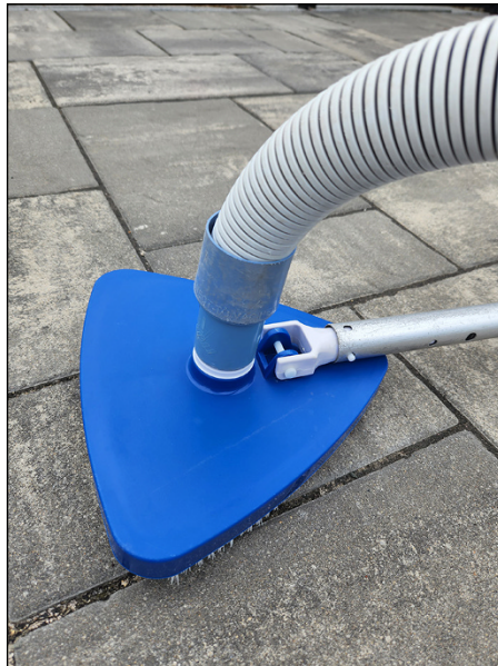
FIGURE 7-3: Attach the vacuum hose securely to the vacuum head.
