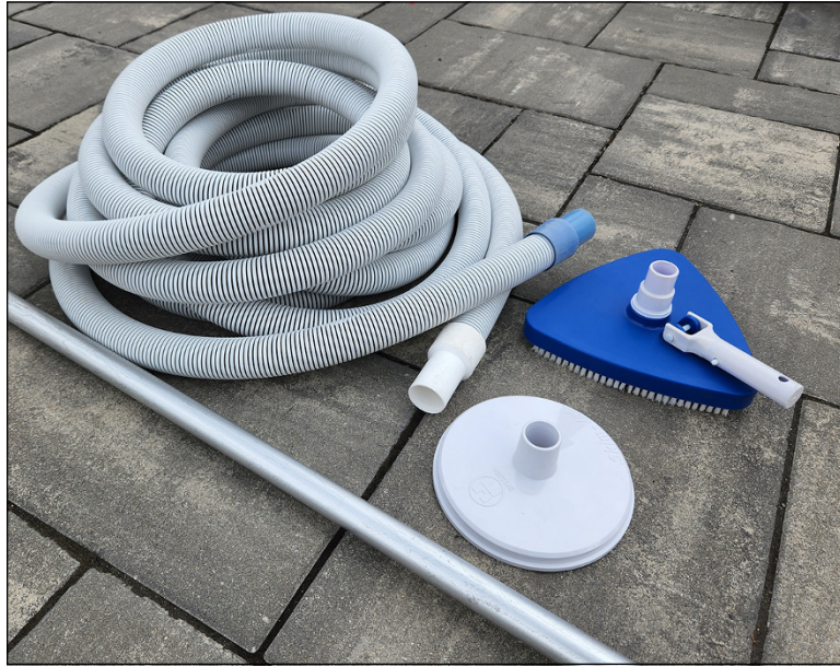
FIGURE 7-1: Tools needed to vacuum your pool: A vacuum head, telescopic pole, vacuum hose, and vacuum plate.
