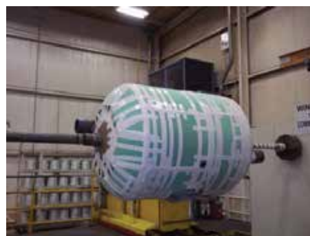
Insulated Vessel at Start of Winding
