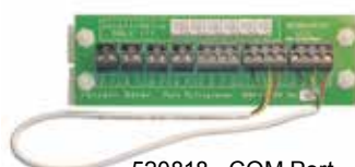
520818 - COM Port Expansion Module
